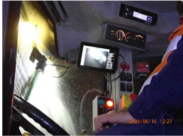
Figure 4: The view of the reversing camera
