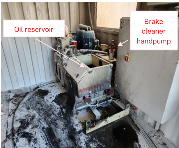
Figure 2 Oil reservoir and brake cleaner handpump
