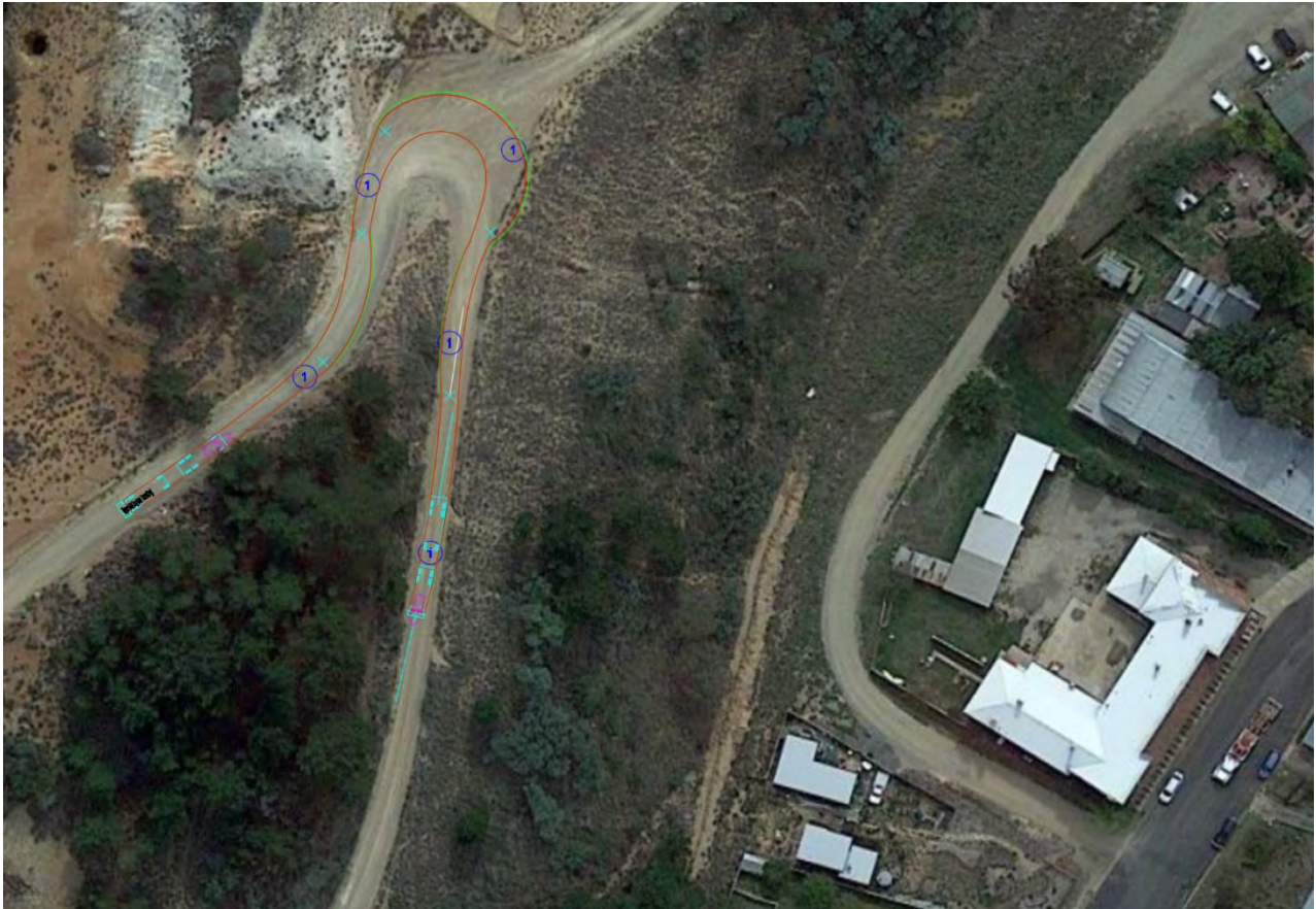
Figure 6: Swept path analysis - Miners Road hairpin turn (right) at 5km/hr (truck and dog combination)
