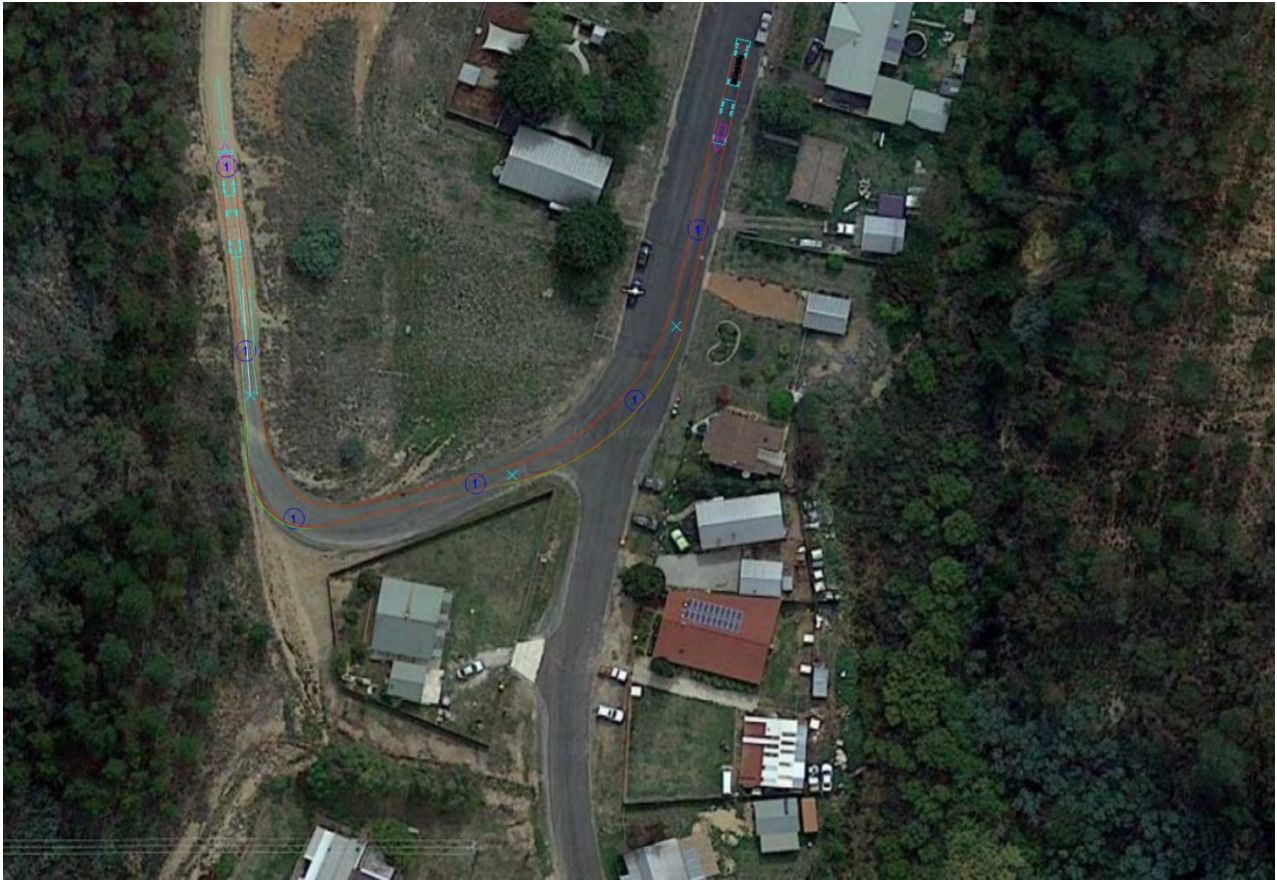
Figure 7: Swept path analysis - Foxlow Street to Miners Road (right turn) at 10km/hr (truck and dog combination)
