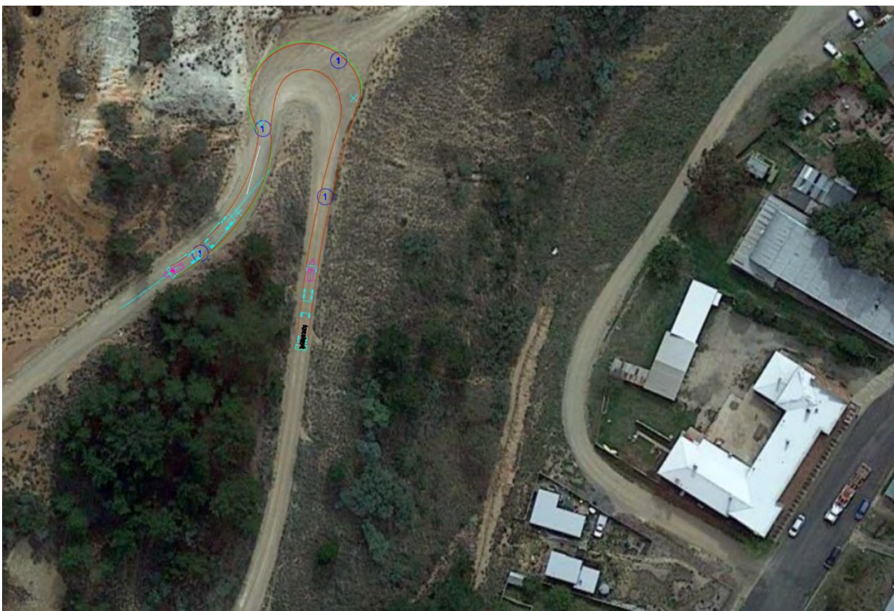
Figure 5: Swept path analysis - Miners Road hairpin turn (left) at 5km/hr (truck and dog combination)
