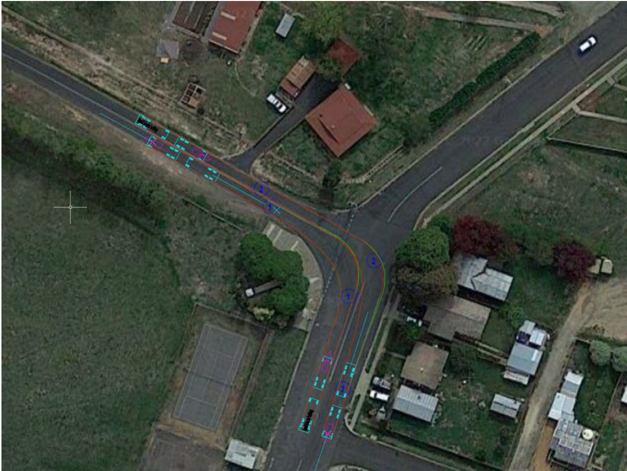
Figure 8: Swept path analysis - Foxlow Street at Captains Flat Road (right and left turns) at 15km/hr (truck and dog combination)
