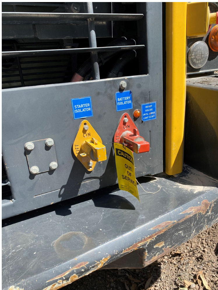
Truck – starter and battery isolators
