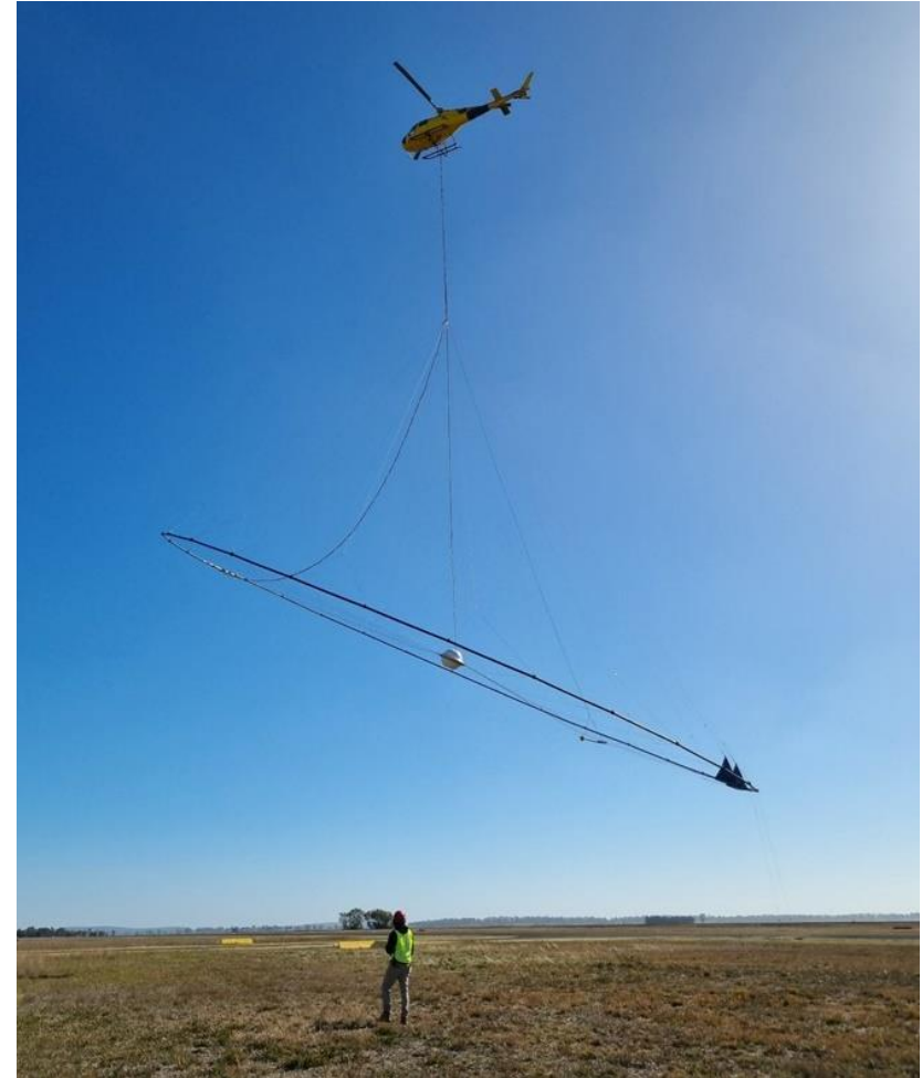
Ground personnel coordinating with pilot whilst landing an electromagnetic sensor.
