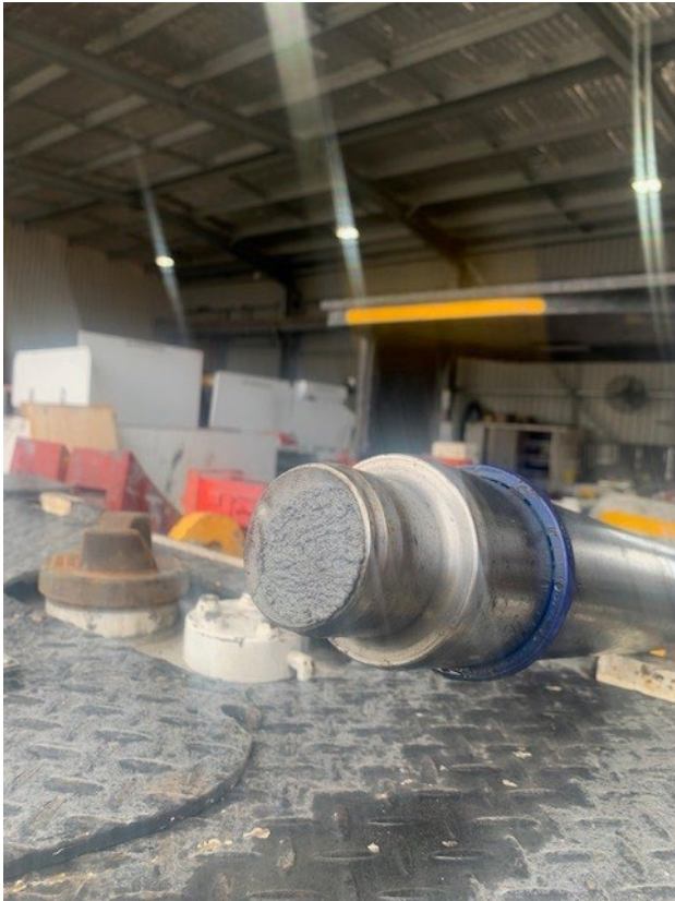
Figure 8: ED7 with duck-bill attachment suffered piston rod end fatigue failure
