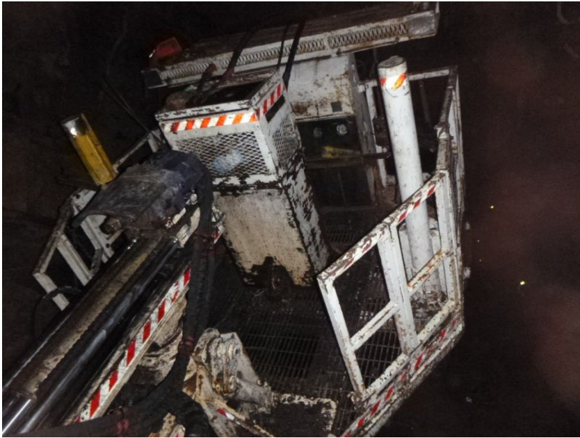
Figure 3: The bolter basket rotated forward with a worker onboard when controls were activated
