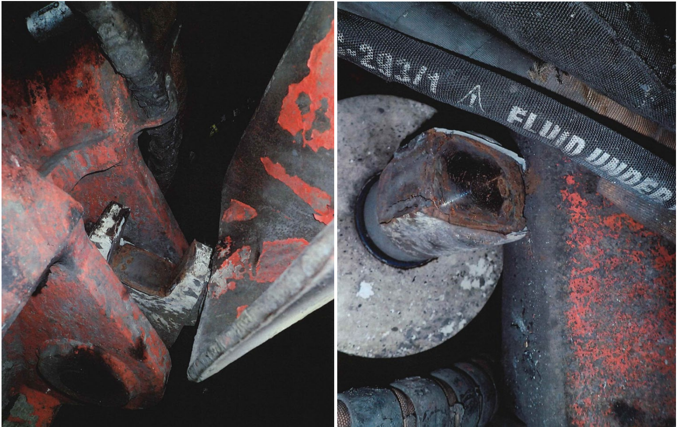
Figures 6 and 7: The ED10 attachment plate crowd cylinder clevis and crowd cylinder rod failed welds
