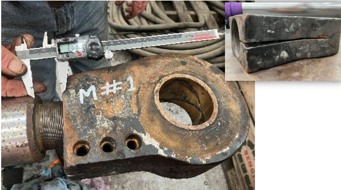
Figure 2: Coaltram CT08 crowd cylinder clevis failure
