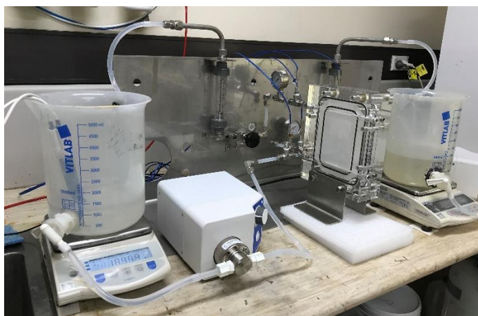
Figure 6: Lab scale flat sheet FO test unit
