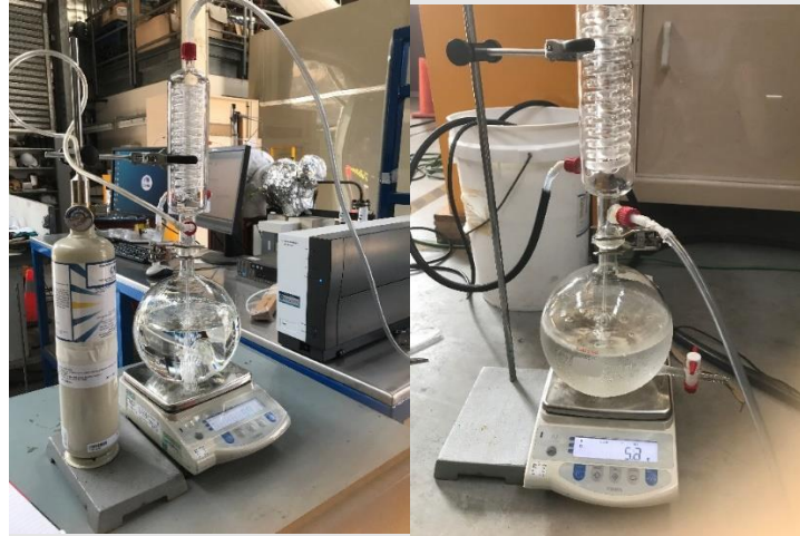
Figure 7: Experimental setup for loading CO 2 in the absorbent solution.
