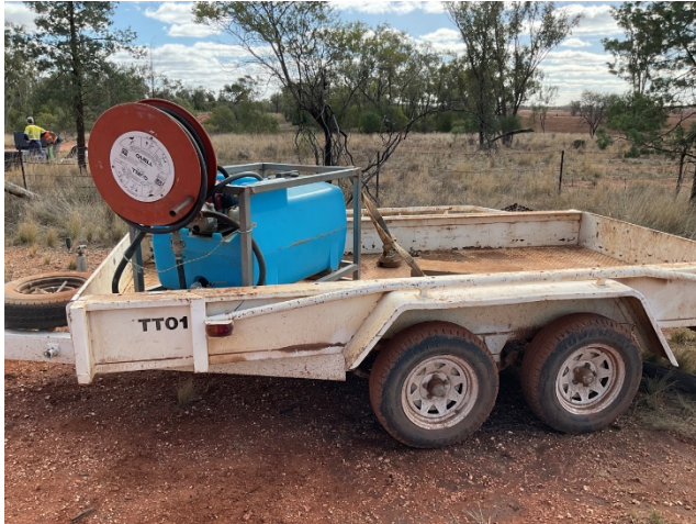
Figure 4 Water tank with fire hose reel in support trailer
