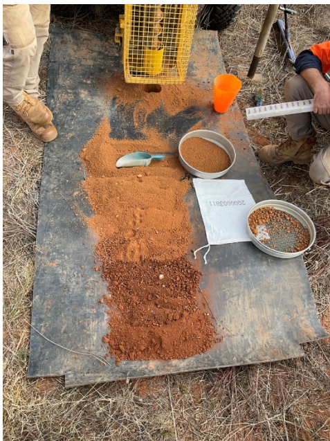
Figure 6 Auger drilling sample collection process
