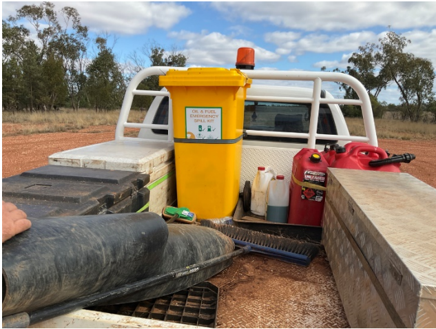
Figure 2 Diesel storage and spill kit on tray of support vehicle
