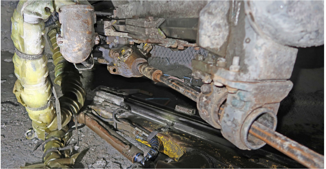
Figure 2: Drill steel inserted into coupling on the right hand drill
