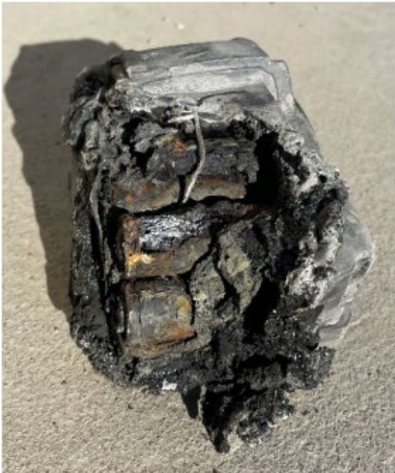
Figure 1 - Damage to battery after being run over
