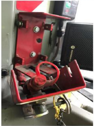
Figure 1 - Actuator panel separated from the mounting bracket
