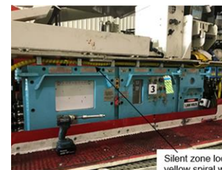
Silent zone loop (protected in yellow spiral wrap)
