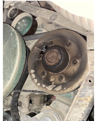
Figure 3: Seized engine idler pulley
