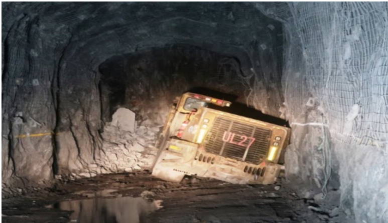
Figure 1 Loader in the 16 level 3400 NPE development drive in the void in the floor
