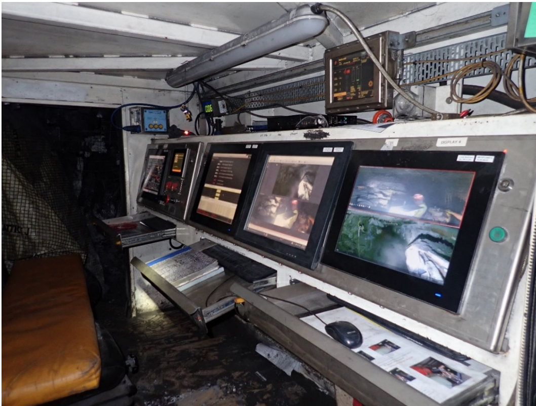
Figure 8: ROS station view from cameras on the miner.
