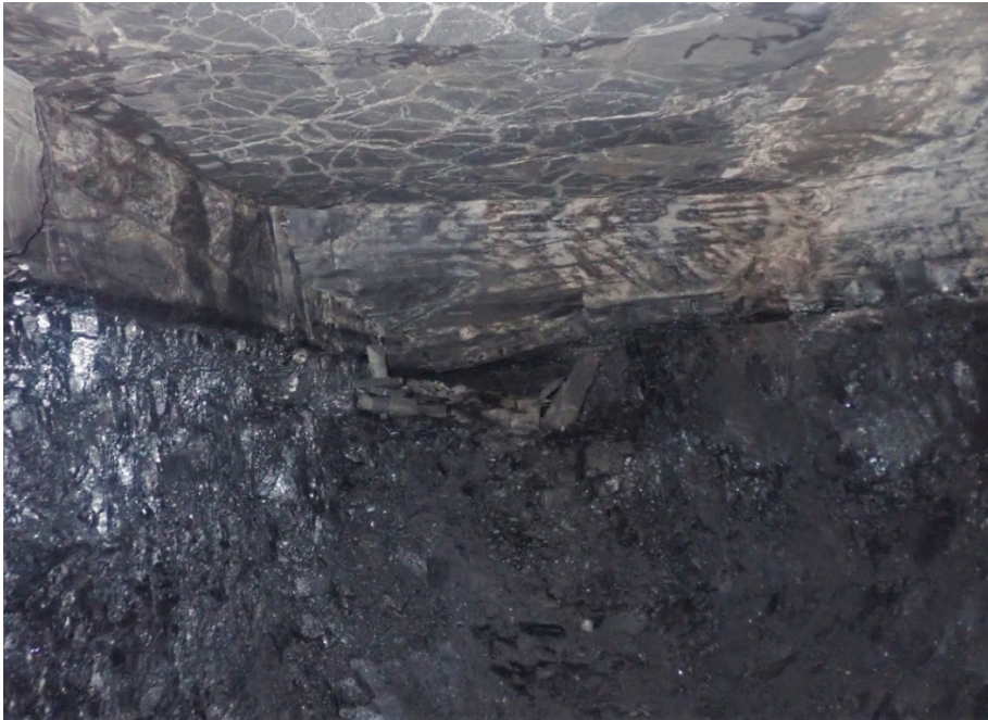
Figure 6: Event 3. View of left-hand side cone after strata support installed
