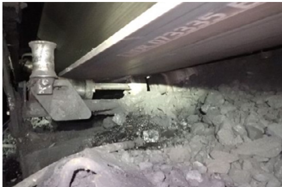
Picture 9. Coal build up under belt.
