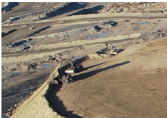
Picture 8. Haul truck (centre left) over windrow.
