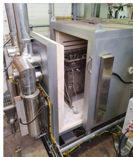
A 1 kW Direct Carbon Fuel Cell developed by the University of Newcastle.
