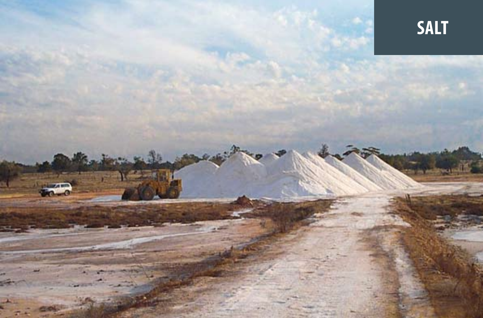
Photograph 18. Raw salt stockpile, Mourquong Basin salt remediation scheme, northeast of Mildura. This salt was obtained by solar evaporation of highly saline groundwater pumped from shallow aquifers in the Murray Basin during salt remediation work. (Photographer J. Whitehouse.)
