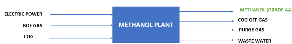
Figure 27: Configuration of Methanol production process using steel mill gases for Scenario 1.
