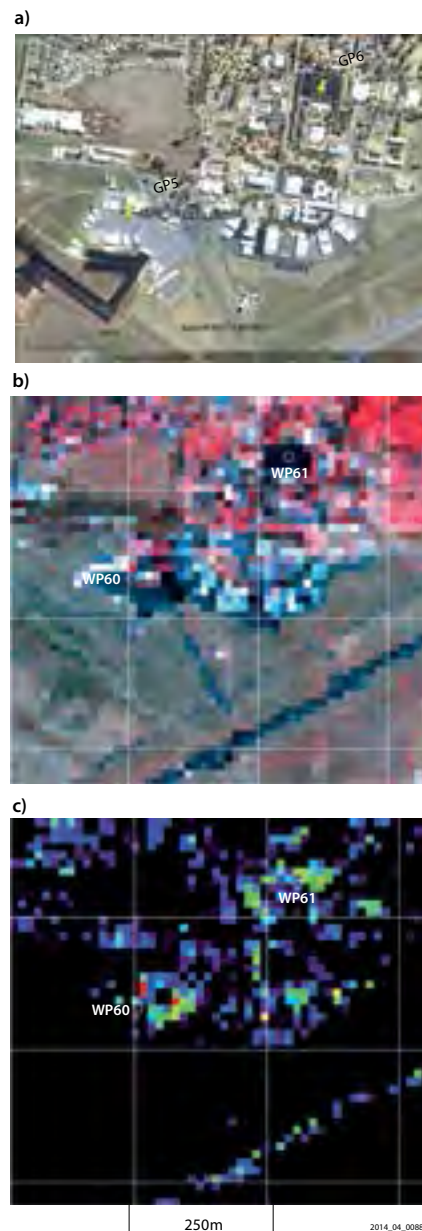
Figure 7. a) Google Earth image of ASTER validation sites at Wagga Wagga Airport (GP5), waypoints WP59, WP60 and RAAF parade ground (GP6), waypoint WP61; b) ASTER False colour image c) ASTER AIOH group content (purple/blue: low to red: high content).
