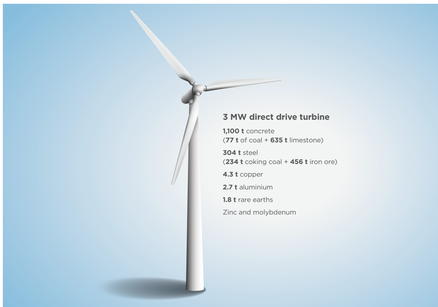
Figure 7: Typical raw materials required for a 3MW direct drive wind turbine
