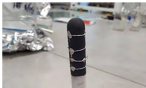
Figure 1. Cathode electrode with a silver wire current collector wrapped around the periphery.
