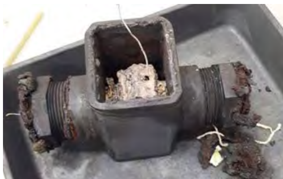
Figure 4. (a) Corrosion data of 316L and 253MA exposed to a slurry (coal + carbonates), (b) post-corrosion photographs, and (c) photograph of the small cell after testing (gland severely corroded).
