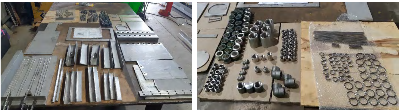
Figure 46. Metal plates and machined parts of the cell unit.
