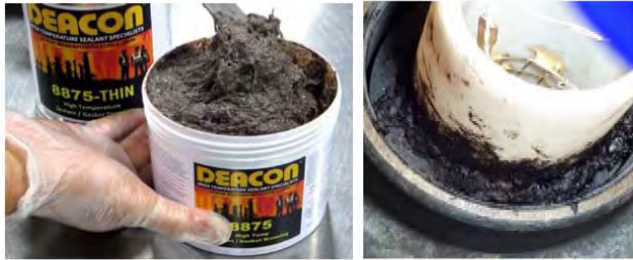
Figure 33. A sealant (Deacon 8875) was applied and cured at 200°C for 2h.
