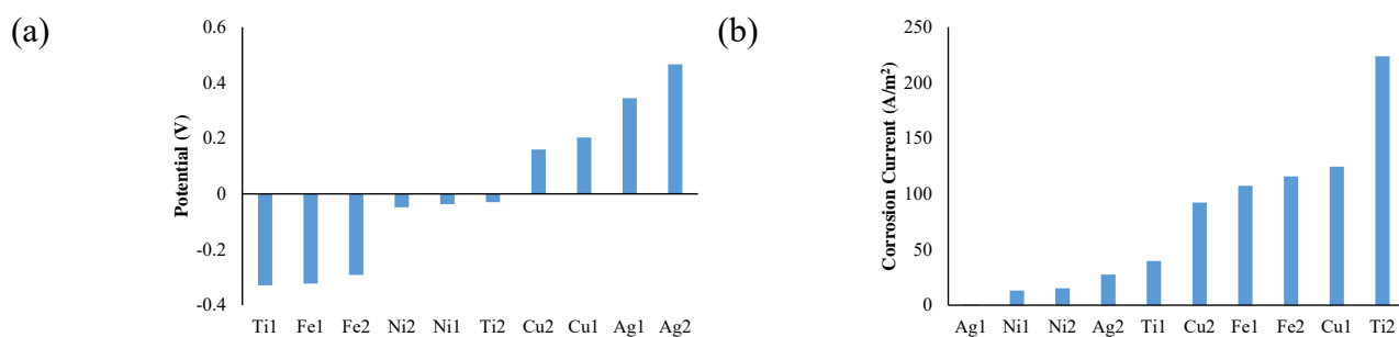
Figure 2. (a) Corrosion potentials and (b) corrosion currents of various metals in the ternary carbonate eutectic at 650°C. Note: 1 and 2 are sample numbers.
