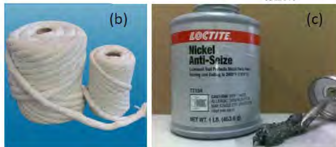
Figure 31. (a) Gland assembly design, (b) Kao-tex ceramic rope, and (c) nickel lubricant.
