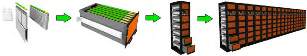
Figure 11 Cells, modules and racks of a Battery System
