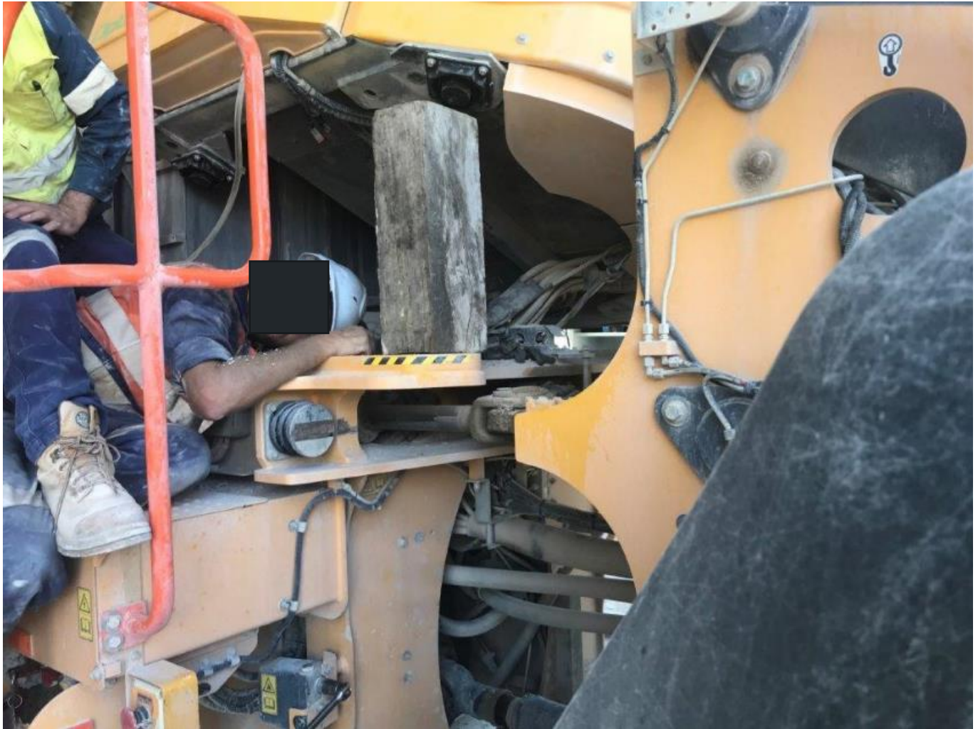
Figure 6 Recovery scene photograph showing the position of the worker on his side after the cab was raised and a wood chock placed by mine workers following his release from the crush point
