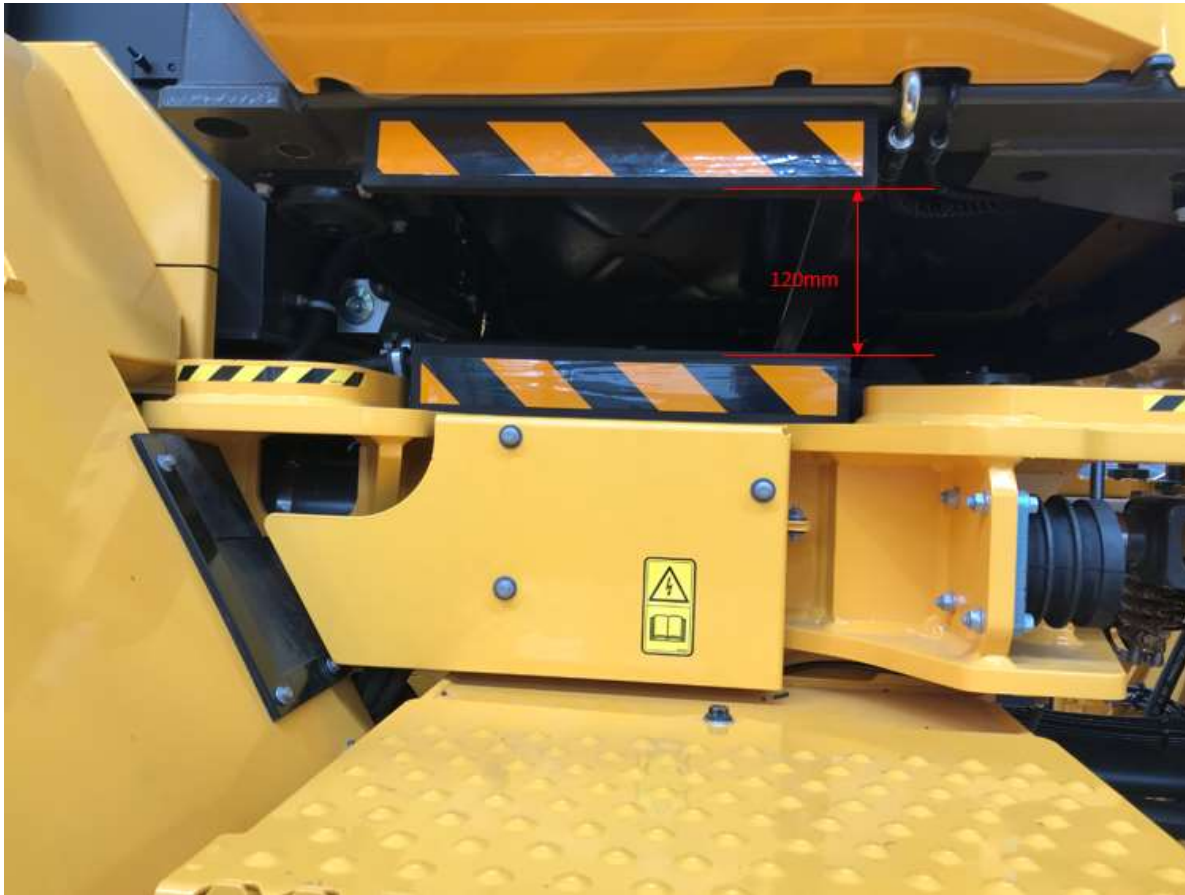
Figure 9 CJD-supplied photograph of two barriers fitted to the underside of a Volvo loader cab to reduce the float gap
