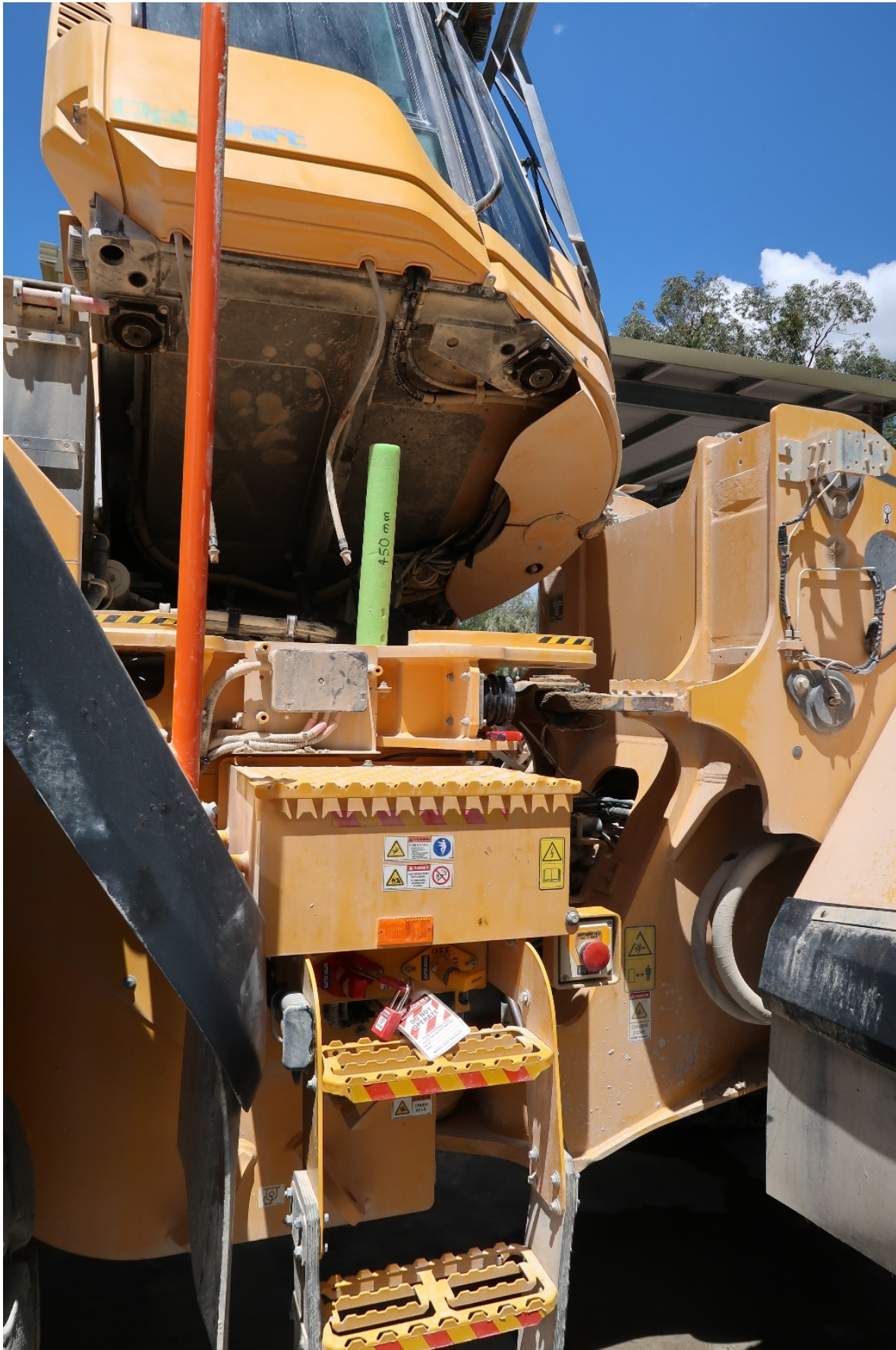
Figure 3 Right-hand side of the loader with cab tilted at position 1 and the lock pin in place to support the cab. A 450 mm green device is placed in the gap between the cab and the chassis for measurement purposes
