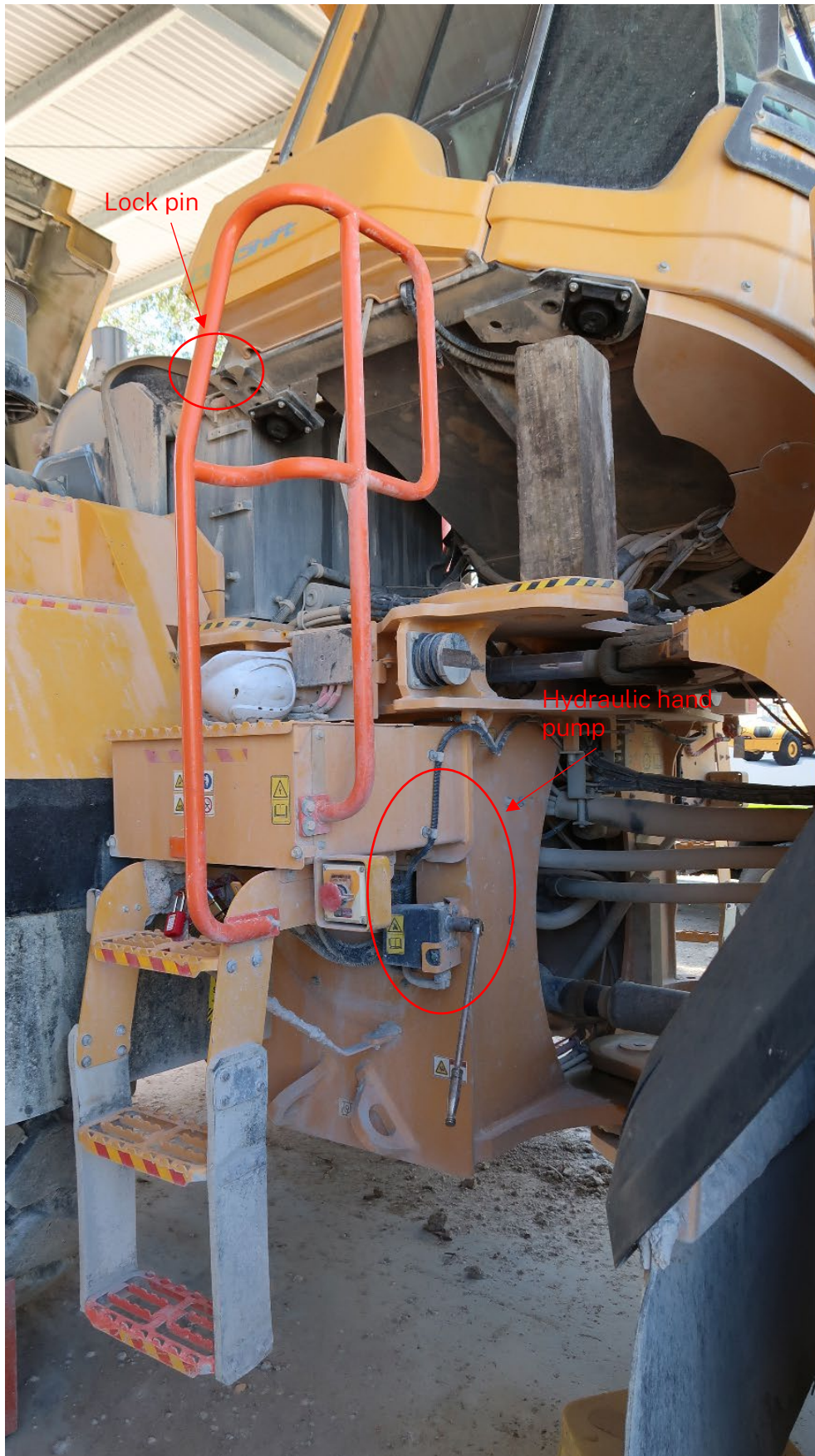
Figure 2 Right-hand side of the loader in the fully elevated position 1 with the lock pin engaged in the Attunga service bay following the incident (Note: the wooden chock was placed following the release of the worker)
