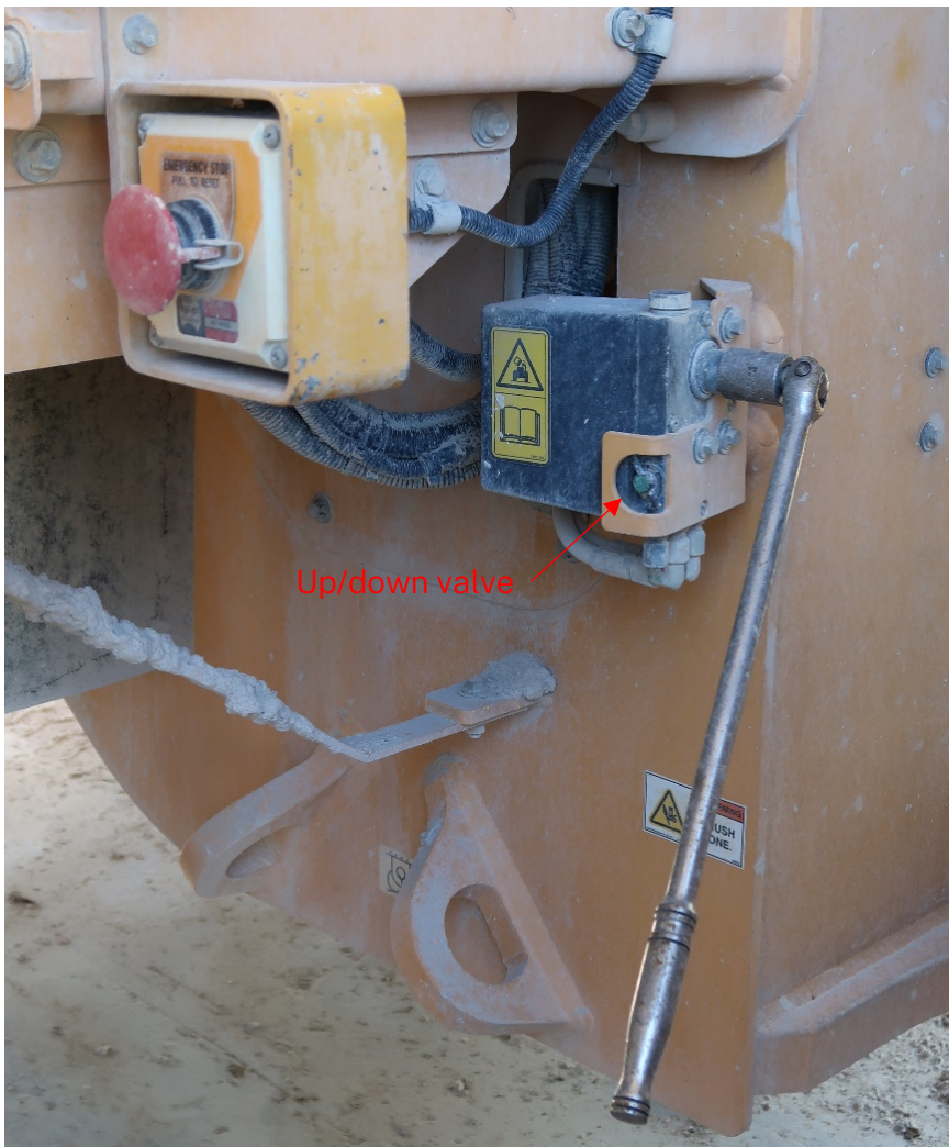
Figure 5 Hydraulic pump and handle used to raise and lower cab
