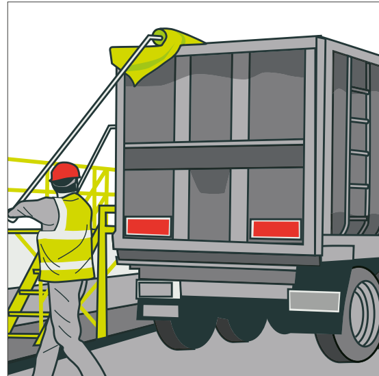
Figure 101. Manual covering system
