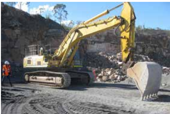
Figure 99. Guardrails are fitted to this excavator to protect workers from falling from the machine during maintenance
