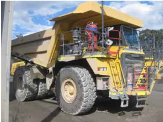
Figure 97. A stairway and platform were retrofitted to this haul truck to increase driver access and egress safety
