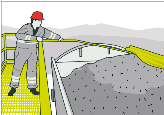
Figure 102. Platform covering system
