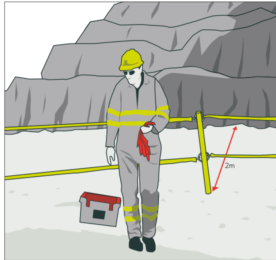
Figure 105. Example of non-weight supportive barriers
