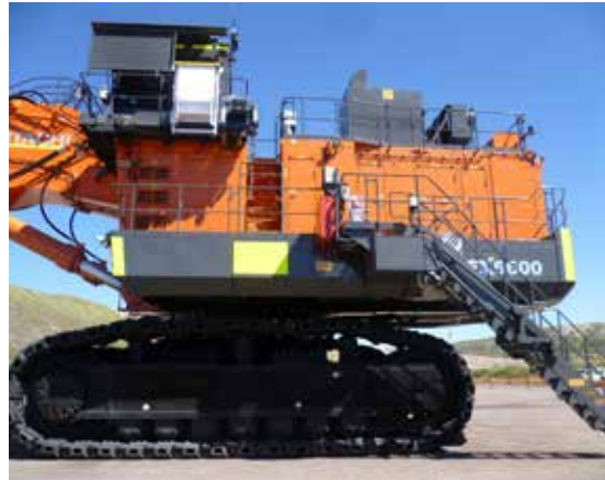
Figure 98. This excavator has a good access system, with platforms, guardrails, kick plates and ladder. The ladder is interlocked so the vehicle cannot be started without the ladder being raised
