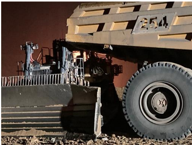
Figure 1 – Haul truck reverses into dozer
