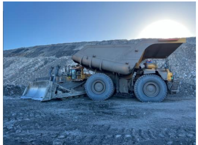
Figure 2 – Haul truck reverses into dozer
