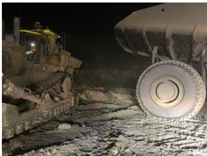
Figure 5 – Haul truck reverses into dozer
