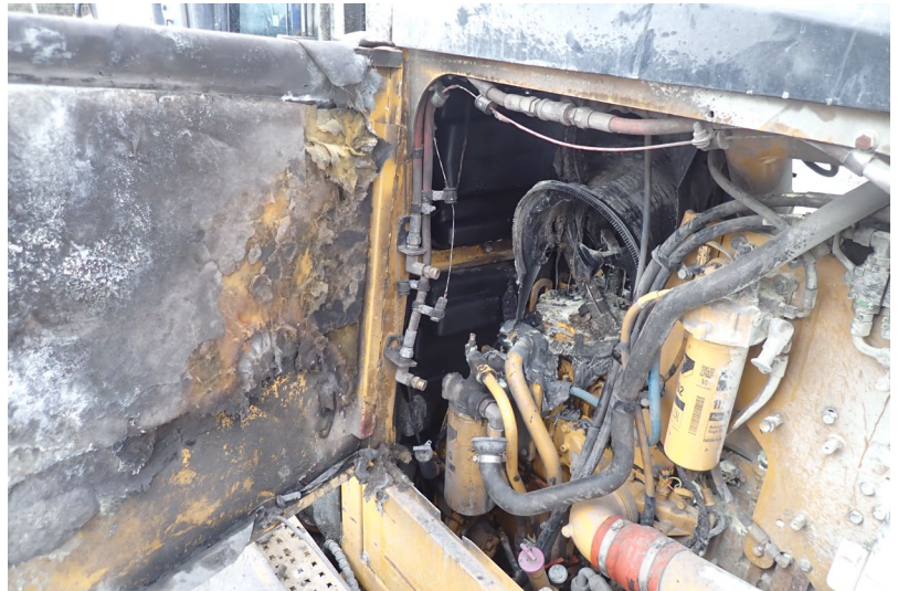
Figure 2: Grader fire damage and location
