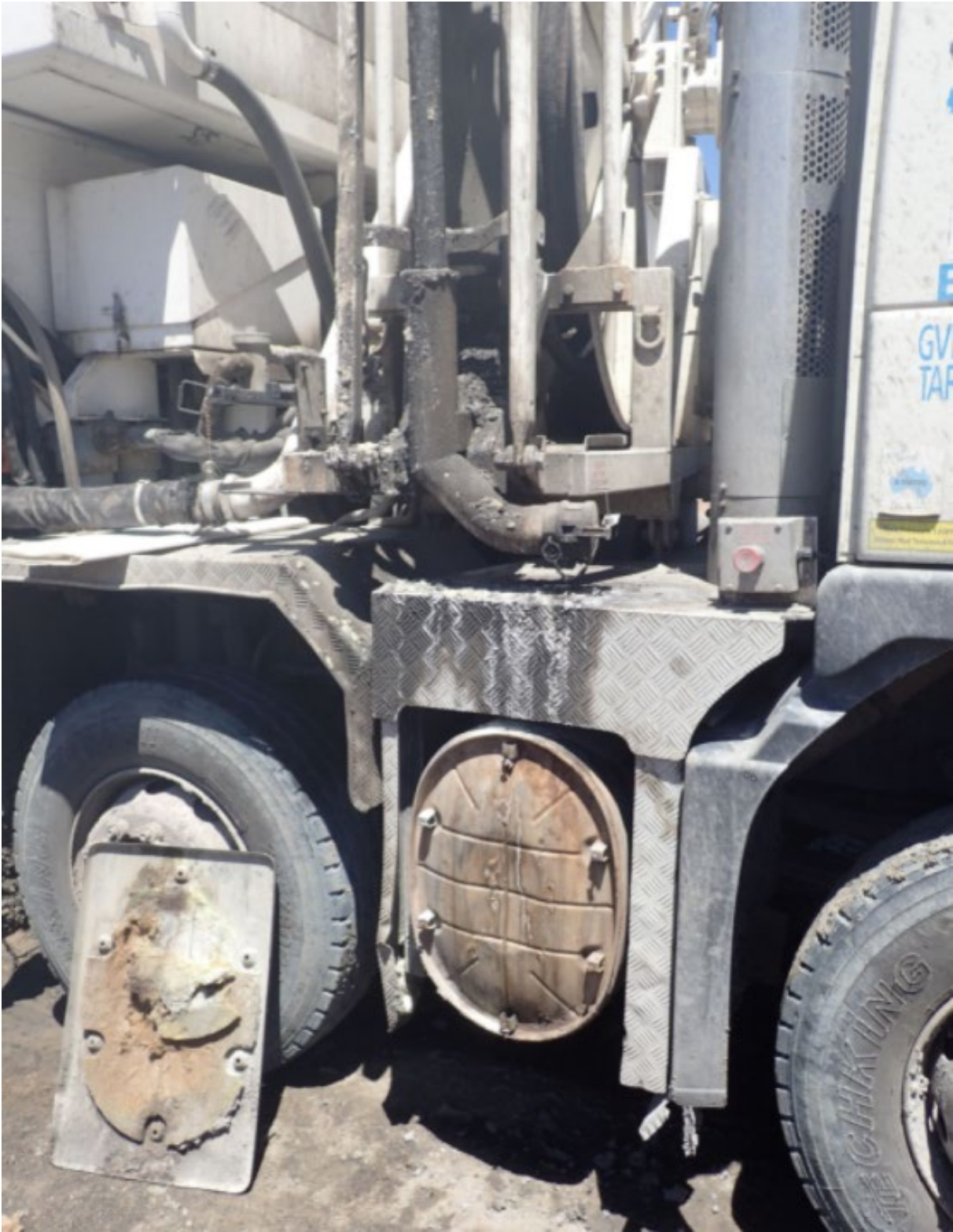
Below: Exhaust components showing area of flames.
