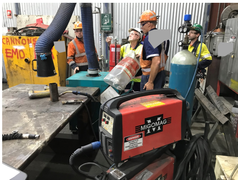
Figure 4: Typical mine hot work bay with LEV unit directly beside work area.
