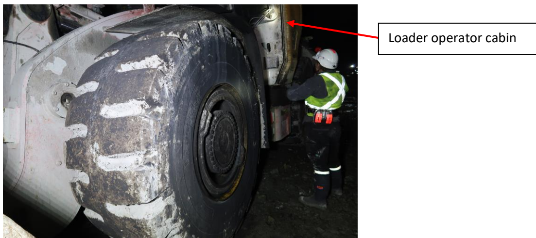
Figure 4: Fire affected position one tyre of loader
